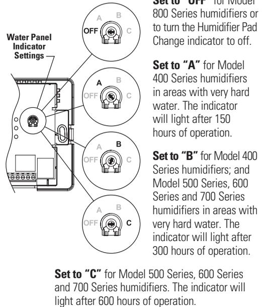
The Model 62 shipped with the Model 800 steam humidifier is factory set to “OFF.” The Model 62 does not have the “Change Water Panel” light on the control. The canister change indicator for the Model 800 is on the humidifier.
