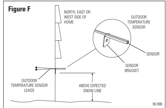
**NOTE:** A convenient way to get the sensor wire outside is to make use of unused wires running to the A/C condensing unit (if applicable). Other ways are to use existing holes for cable TV lines, telephone lines, A/C lines, etc. Read all equipment instructions beforehand for possible conflicts and warnings.
