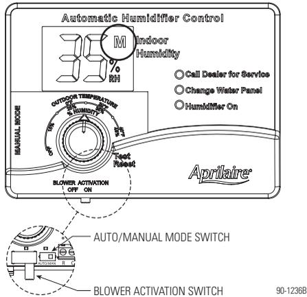
**NOTE:** If control setting was changed between Automatic and Manual mode, power to the control must be cycled by removing then reinstalling the R wire.
